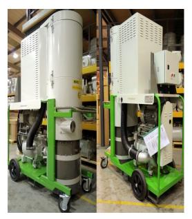
The unique filter design enables air to flow at these rates through the machine whilst offering very high levels of protection and filtering. The large surface area clearflow filter permits excellent air flow whilst trapping dust. The H14 HEPA filter then offers filtering and protection collecting 99.995% of debris at MPPS (Maximum Penetrating Particle Size).
