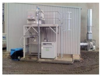
They have been sized for a single operator using a 76 mm bore hose and tool, carrying out heavy duty vacuum cleaning and bulk spillage removal of the wood based biomass materials.
